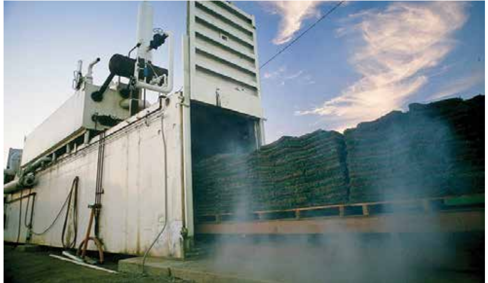
SOUTHLAND SOD FARMS' SOD is placed onto a rail car, which is pushed into the vacuum chamber. As the vacuum is drawn down, the sod cools evenly throughout the pallet. This process reduces the sod pallet temperature to about 43 degrees in less than 20 minutes.
